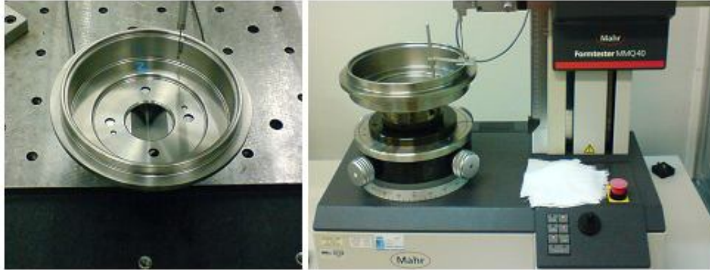
Figure 31. Measurement (left) and calibration (right) of a brake drum.
